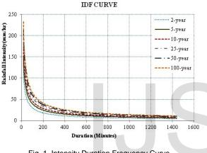
Fig. 1. Intensity Duration Frequency Curve
