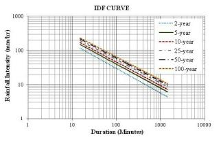
Fig. 2. Intensity Duration Frequency Curve in log paper
